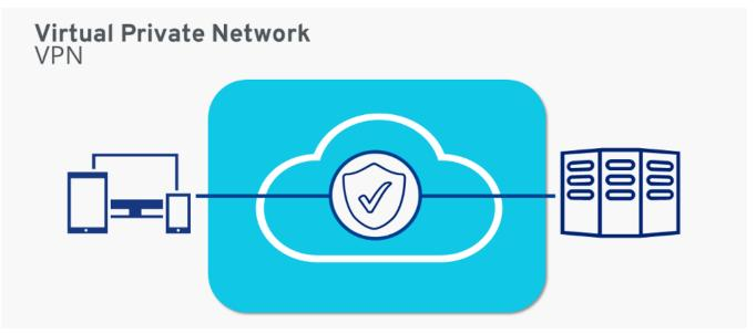
A VPN connection creates a secure tunnel through the internet between the employee's PC and the company's server infrastructure.
